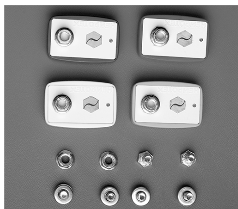
Fig. 1. Sensors for “Kolibri” electromyography (Neurotech LLC, Waukesha, WI, USA) and the clamping screws.
