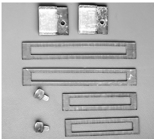
Fig. 3. Polymer plugs created by 3D printing, and horizontal plates with rectangular holes and fixing screws.
