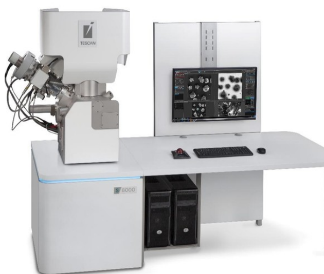
Fig. 2. TESCAN Mira 3 LMU scanning electron microscope (TESCAN, Czech Republic).
