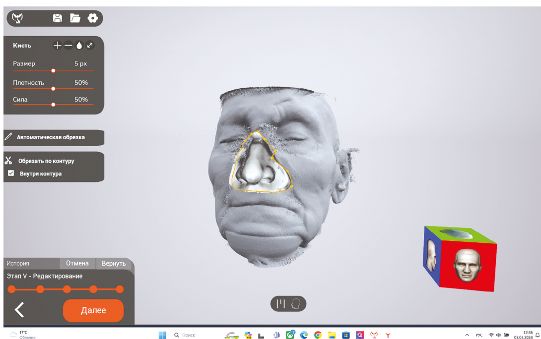
Fig. 3. Automatic adaptation of the virtual nose model to the tissues of the prosthetic bed in the Phoenix 3D program.
