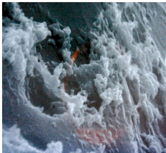
Fig. 3. Increased surface relief of Ftorax acrylic resin denture base. \times 400 . Scanning electron microscopy (SEM).
